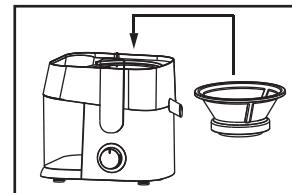
(Note: When assembling, please install Juice Tray first, and then install the filter unit. When disassembling, please remove the filter blade first, then remove Juice Tray.)
