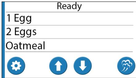
3. When the unit reaches proper heat, it displays the **Ready** screen and shows the list of the first three menu items in alphabetical order.
