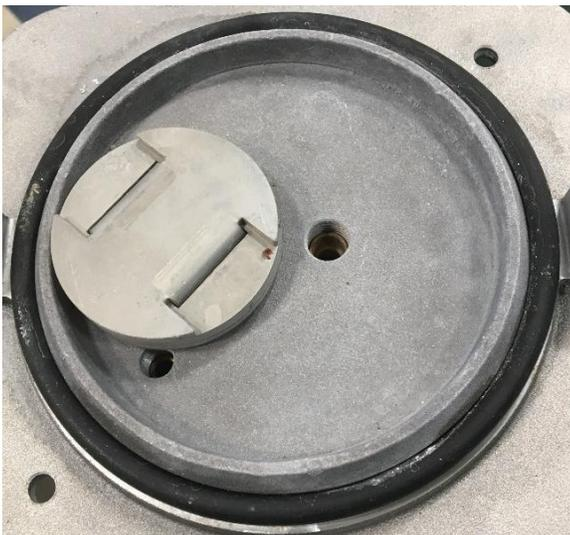
Figure 7. Properly Lubricated O-Ring
