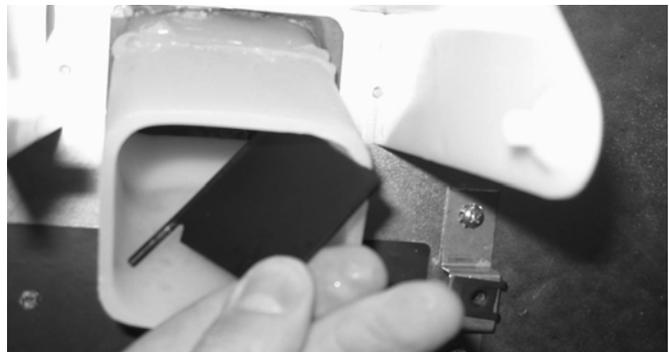
7. Pull the paddle wheel guard from the holes inside the ice dispense snout.
