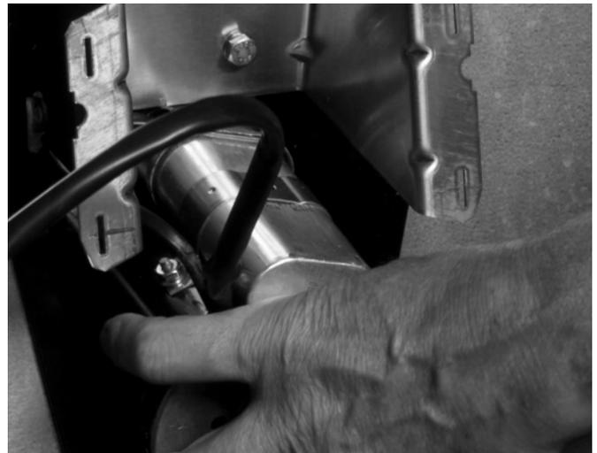
5. Grasp the gearmotor as the second pin is removed.
