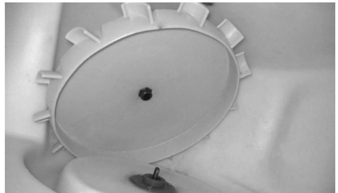
4. Slide the paddle wheel from the motor shaft and remove.
