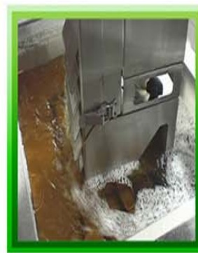
Put the machine into fryer, press the red button. Machine itself time 15 min.
