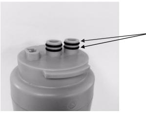
Lubricate all **four o-rings** with a good food grade silicon lubricant prior to installing the filter head.
