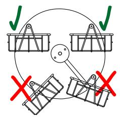
The baskets should be loaded evenly to ensure a smooth balanced operation. Take care that baskets are more or less level when loaded. Uneven loading may cause the baskets to fall against other baskets or sides of the unit and cause damage to the appliance.
