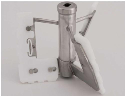
Removable and flexible agitator blades touch the horizontal cylinder to obtain a consistent and homogeneous mixing . Thermal impermeable , non-adhesive , spring-loaded POM scrapers , remain the cylinder clean and freeze evenly , to give a beautiful finish gelato presentation .
