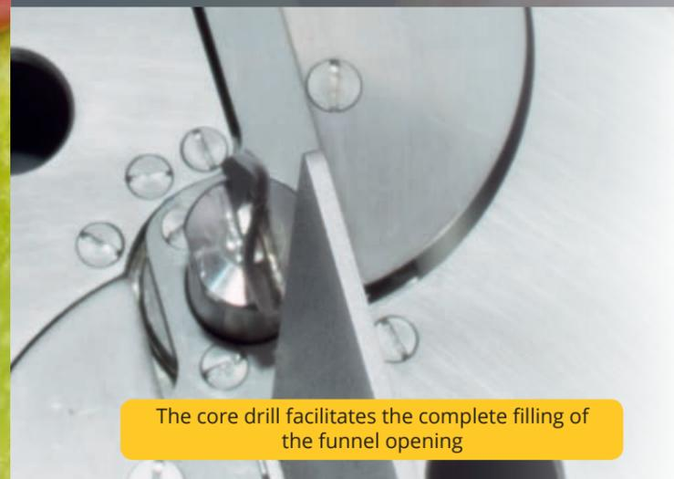
The core drill facilitates the complete filling of the funnel opening
