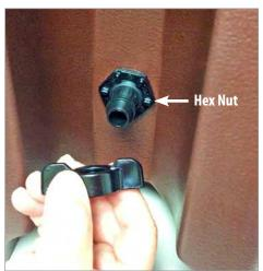
Now with the wing nut loose, use the wing nut as a tool to turn the hex nut to the LEFT to loosen so that the spout can be removed from the body of the beverage server.
