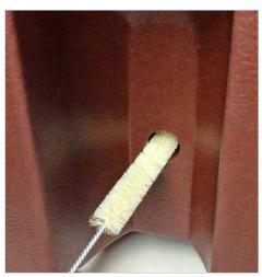
Use the bottle brush to also clean the spout drain port in the body of the beverage server. Rinse and dry.
