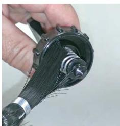
Clean the coil area on the faucet lever stem as well as around the inside area of the lever cap.
