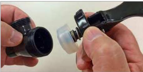
Next, disassemble the faucet by turning the faucet lever assembly COUNTER-CLOCKWISE until the lever section comes out of the body.
