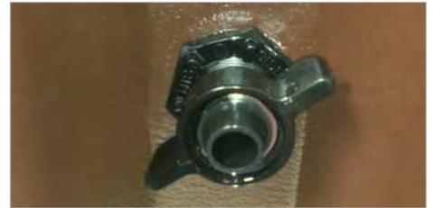
With the wing nut still on the spout, put the metal C- ring back on, placing in the groove just ahead of the wing nut to prevent it from coming off.
