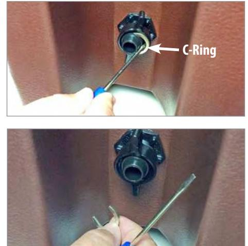
Locate the metal C-ring and with a small metal screwdriver, carefully slide it out of its groove on the spout end.
