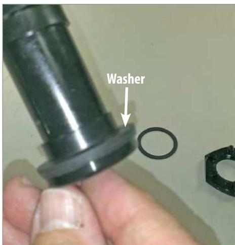
Place the rubber seal washer back on the spout sleeve in the groove on the flared end.
