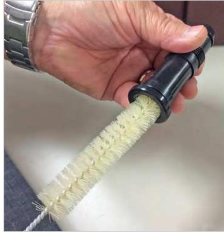
After removing the seal washer for cleaning, take a small bottle brush (can be purchased at Harbor Freight) and using warm water and mild detergent, thoroughly clean the spout sleeve, rinse well and dry.
