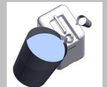
Mix the supplied ConvoCare Kconcentrate with soft water in the empty ConvoCare rinse aid canister. Follow the instructions in the user manual on mixing the ConvoCare rinse aid in the canister.
