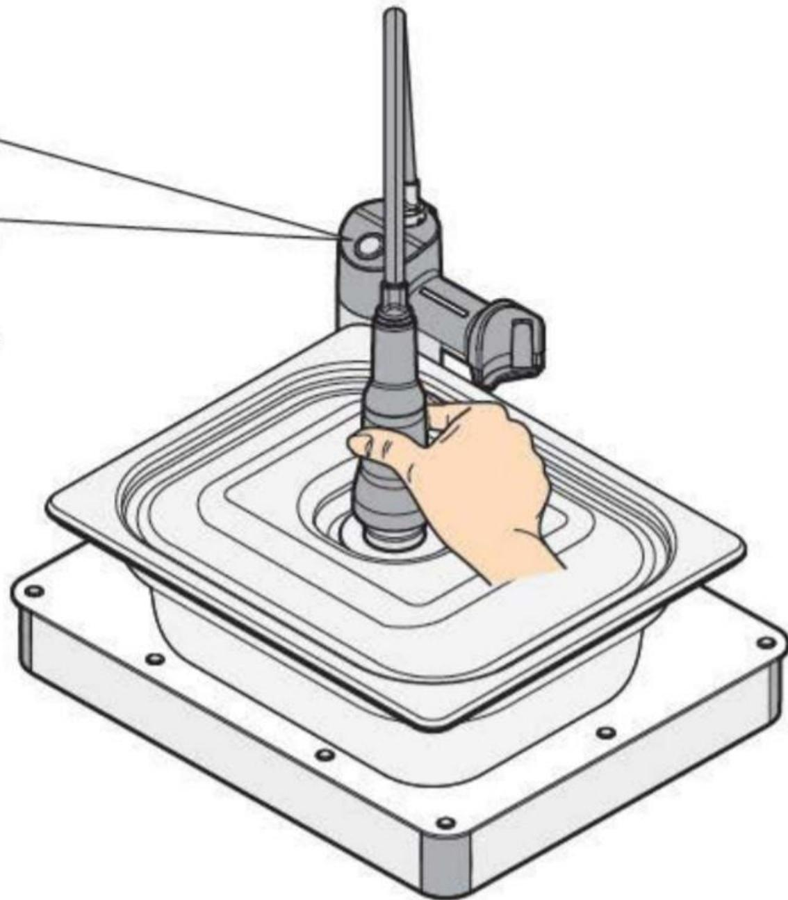
Wearing rubber gloves and goggles, spray UNOX SPRAY&RINSE on the steel parts. Do not spray the product on the suction pad as this may cause damage over time.
