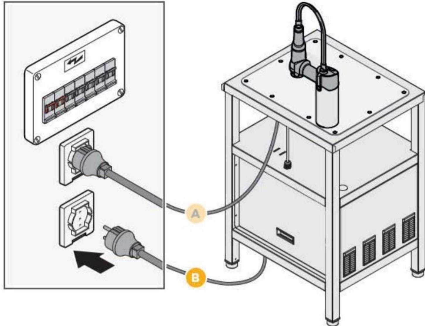
If, after making all electrical connections, the compressor does not work, remove the panel at the back ▶ 15 and check that the built-in compressor switch is set to "ON"
