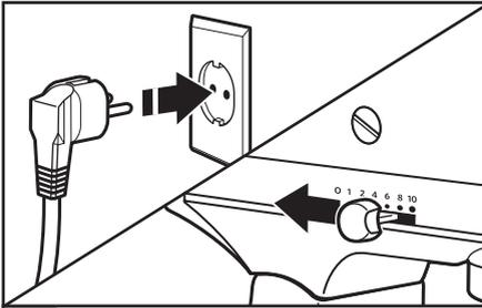
**1** Plug Stand Mixer in proper electrical outlet. Always set speed control lever on lowest speed to start, then gradually increase speed to avoid splashing ingredients. See chart below.
