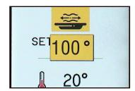
This function allows to bring product cooked previously back to temperature by setting a correct mix of temperature and humidity.
