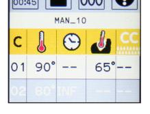
After the program has been started by the "START/STOP" key, the probe's actual temperature (23°C) will increase until reaching the settled value (65°C).
