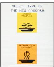
The "REFRIGERATED HOLDING" function allows to hold food at a temperature between 0°C and 30°C.
