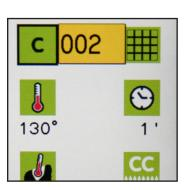
NOTE: if a temperature value for the core probe is set automatically the (ex. 38°), the time disappears. This happens because it is the reaching of the probe temperature that determines the end of the cycle.
