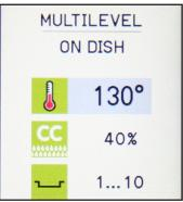
To set the temperature, select the corresponding line for this parameter and press "ENTER" using the Touch Screen or scroller.
