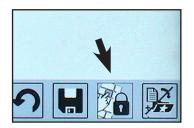
The "SERVICE" screen brings together a series of "service" functions, which can be accessed by selecting the "Service" icon using the Touch Screen.
