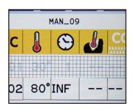
**NOTE:** once the program has started, you can change the set values while the device is running (always using the Touch Screen, or knob, and the "ENTER" button). Once the program is over, the modified values remain in the local memory; to save them select the icon "SAVE" (see chapter "Memorization of a program").
