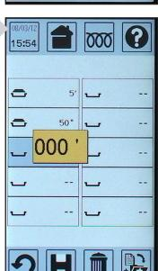
**NOTE:** the setting of the "core probe" for a plate or a level automatically blocks the probe icon on the others in which only the time modification will be possible.
