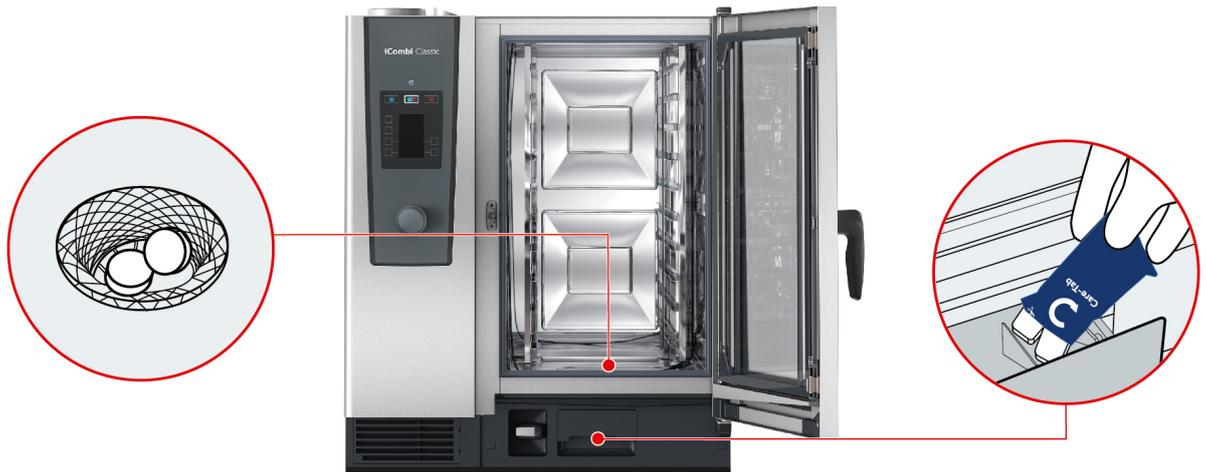
8. **⚠ WARNING! Danger of chemical burns! Wear a face mask and chemical-safe gloves for reliable protection when handling Active Green cleaner tabs and care tabs.** Unpack the displayed number of Active Green cleaner tabs and place them in the drain sieve of the cooking cabinet.
